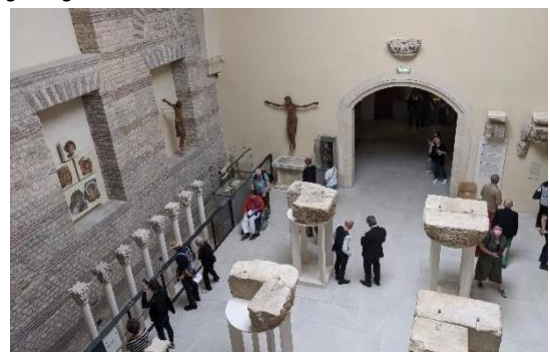
Figure 36: raised platform in historic space for accessibility. Power and mechanical systems located discretely below platform.
