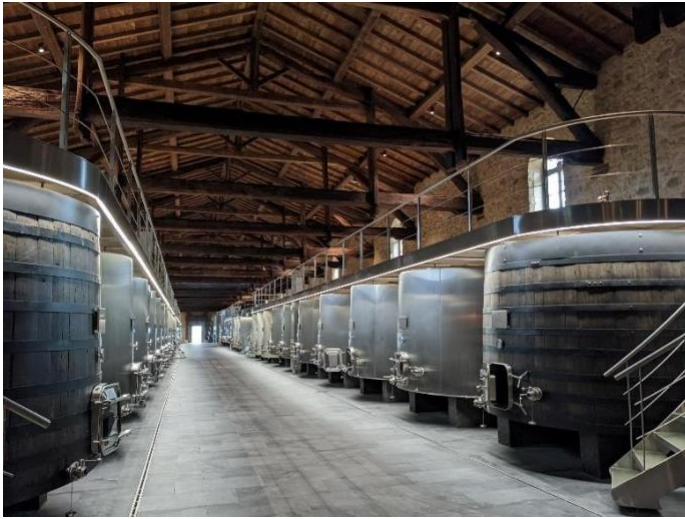
Figure 20: upper level for fermenting of wine in concrete and stainless steel drums
