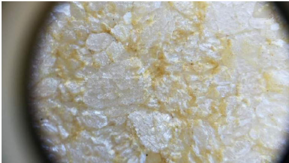
Fig. 7.2 Closeup view of marble after first pass of adhesive removal with dry ice. 10X microscope view. Constance Lai. August 14, 2018.
